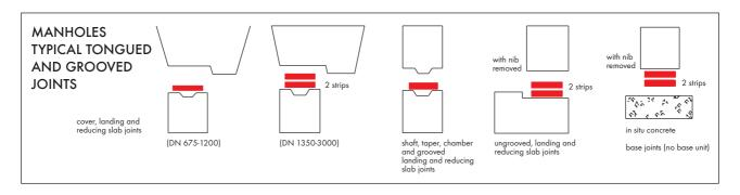
AQUASTRIP cross-sections and sizes are designed to fit the tongued and grooved, rebated or ogee joints of all makes and sizes of precast concrete manhole and inspection chamber sections and slabs to BS 5911 Parts 2 & 200, and BS 5911-1, -3 & -4 and BS EN 1917.
